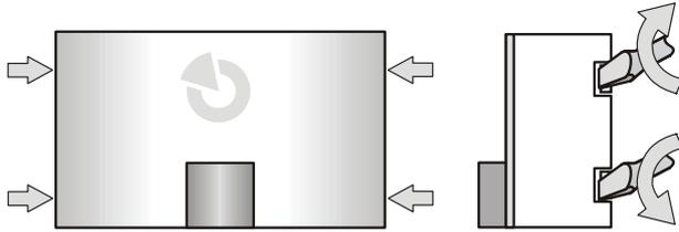
1. Open the indicator cover by loosening the four tabs by twisting them in the direction indicated by the arrows using a suitable screwdriver.
