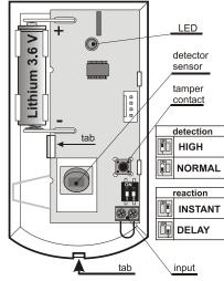
appliances etc. being positioned within its detection area. Moving objects with a temperature close to that of humans such as curtains moving above a radiator, and pets should also be avoided. Detectors should not face windows or spotlights or be near fast-moving air e.g. near ventilation fans or open windows or doors. There should also be no obstacles blocking the detector's "view" of the protected area. Keep the detector away from metal objects which could interfere with radio communication.
