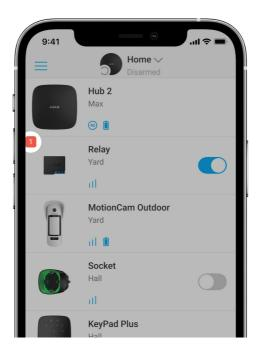
In case of Relay fault (e.g., no Jeweller signal between the hub and the relay), the Ajax app displays a malfunction counter in the upper-left corner of the device icon.
